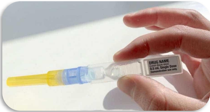
RFID/NFC instrumented prefilled syringe verifies time, place, medication of each injection
