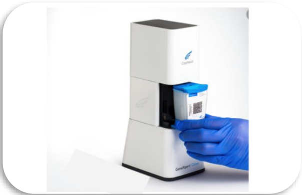
Blood analyzer with RFID-enabled test assay cartridges for authentication & verification
